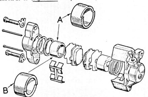
In the case of the Sprite, the cutaway part of the piston faces downwards, as shown at 'B'.
